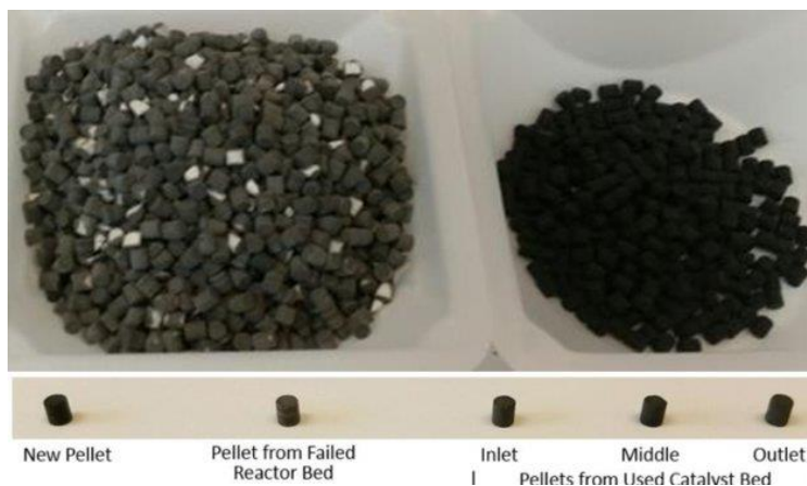
Figure 4. Top: Left: The 2015/spent catalyst that was damaged; Right: New/unused catalyst; Bottom: Ru/Al 2 O 3 pellets that were characterized.
